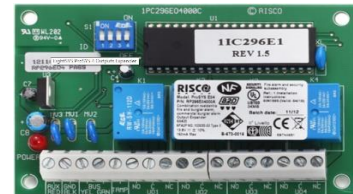
4 x 3Amp Relay Module
