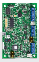
The Voice Module gives LightSYS panels the ability to verify alarms or reduce false alarms via two-way voice communication with the Central Station, for PSTN only installs. The Voice Module also add voice annunciation for zones & system state.
