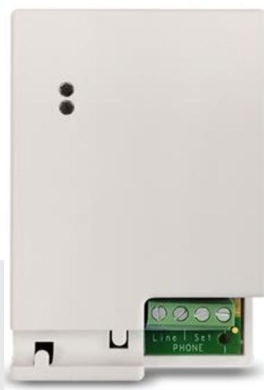
The plug-in PSTN module enables the panel to communicate with a central station (ARC) using common format protocols (SIA, Contact ID). The PSTN module can be used as a primary communication channel or as a back up to the Cloud connection, in case of communication failure. The module should be plugged into the GSM/PSTN module slot on the LightSYS+ panel. In installations that require both PSTN and GSM modules, the GSM module should be installed on the COB (Cellular on Bus)
