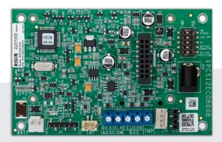
The Cellular on Bus Module (COB) enables the installation of a cellular communication module outside the Control Panel along the system bus, allowing flexible positioning of the cellular module for optimal cellular signal level. The COB is an interface board, on which either 2G or 3G modules can be plugged.
